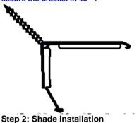
Position head rail at an angle so that it is hooked to the front of the bracket. Then push it upward to snap into the bracket.
