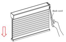
Note: the control cord cannot be too tightened / taut when installing due to its own system character. There should be no obstruction when the shade going down.
