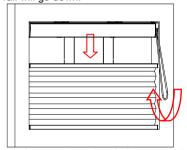
Go on pull the control cord as below arrow direction, once the middle rail reach the bottom, the middle rail & bottom rail will go up together.
