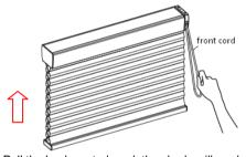
Pull the back control cord, the shade will go down automatically, till it fully close.
